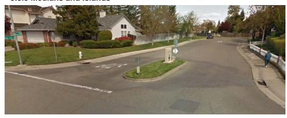
A median is the portion of the roadway separating opposing directions of the roadway, or local lanes from through travel lanes. An island is defined as an area
